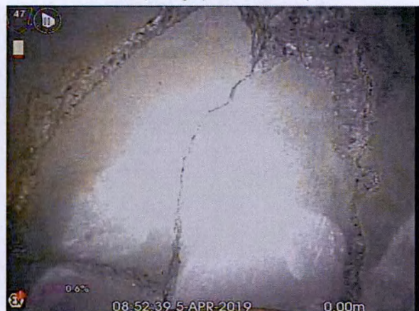
S7X_ca062aaf-6af5-4bed-ad91-987a9282a6d7_20190405_095147_073.jpg, 00:00:40, 0.00 m Fracture spiral from 9 o'clock to 3 o'clock
