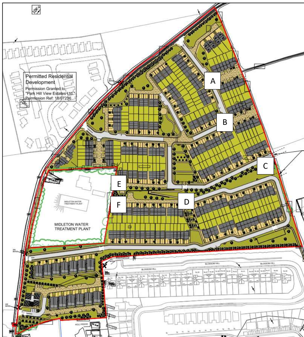
Figure 6.10 Plan of site showing potential vulnerable locations during a pluvial exceedance event
