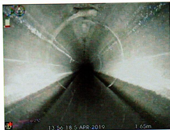
S12X_a4c78e13-8fa1-48da-99c7-0acaecf3be4c_20190405_145527_027.jpg, 00:00:12, 1.65 m Water level, 10% of the vertical dimension
