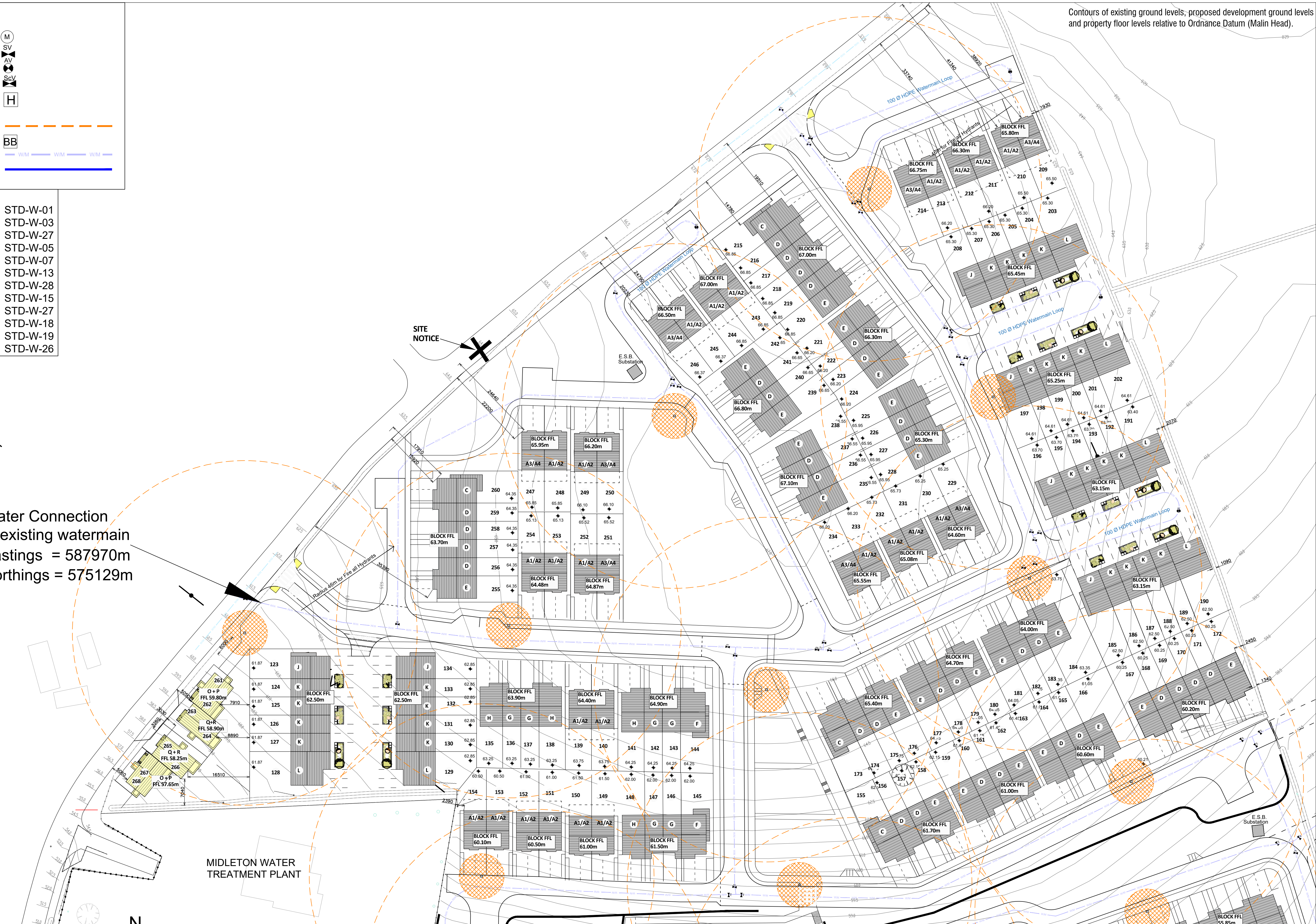
PART SITE PLAN - NORTHERN SECTION - WATERMAIN LAYOUT Scale 1 : 500
